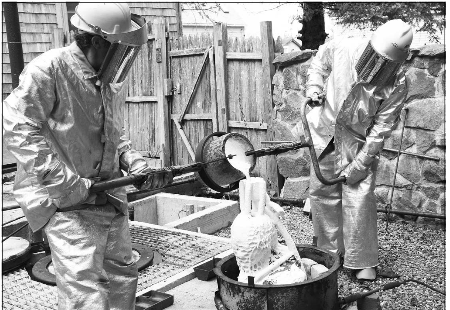
POURING molten bronze into the shell mold for a section of the mermaid sculpture to be placed on the Eastport seawall are Bill Labbadia (left) and Dick Klyver. The casting was carried out at Klyver's bronze foundry in South End on November 15. (Edward French photo)
